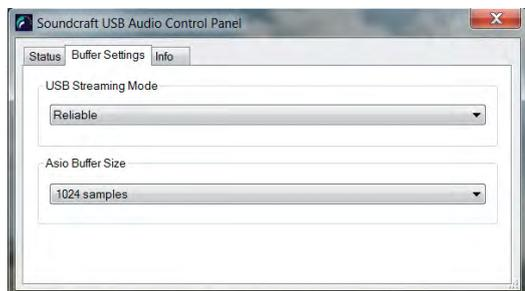
Recommended buffer size will vary depending on application, however higher buffer sizes should be used when monitoring from the DAW is not necessary. For most live recording applications, a standard buffer size of 1024 samples is enough to ensure reliable operation and clean audio.
