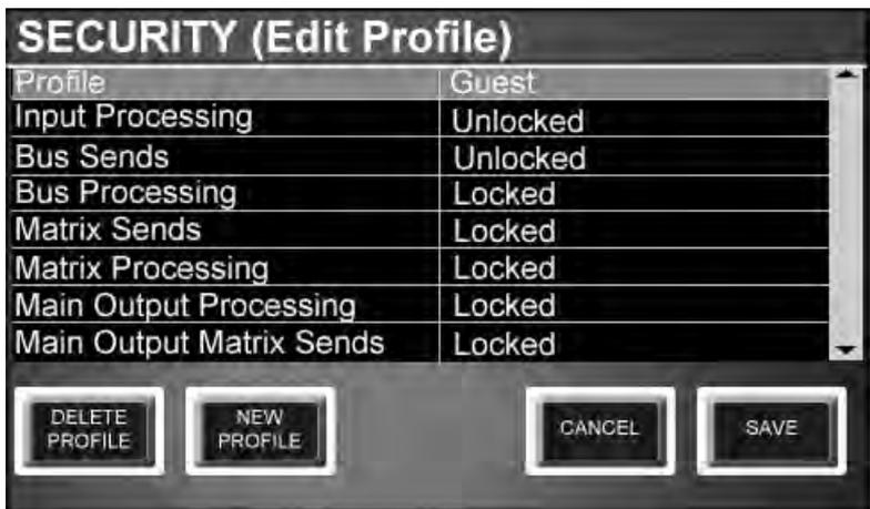
NOTE: If a Cue recall will change an aspect of console functionality that is locked, but Cue List functionality is not locked, the Cue will still be recalled as normal.
