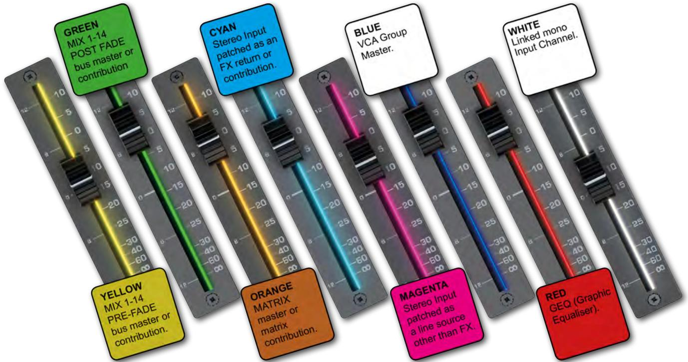
Several different functions can be assigned to the console faders, so it can be easy to lose track of which function is currently being controlled, especially when grabbing a fader in a hurry. The main principle of FaderGlow is to indicate the current fader function with colour, so more immediate recognition is possible. Soundcraft FaderGlow is fitted to all console faders that can change their function.
