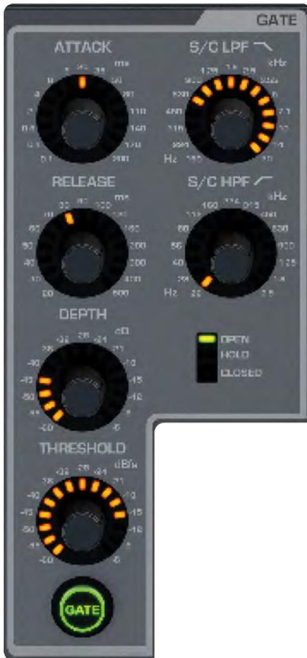
A Gate is a threshold-driven gain reduction process normally used to attenuate a signal when its level falls below the Threshold. Setting the Threshold just above a noise floor or background noise, for example, will allow the Gate to attenuate the source during periods when the main input (voice, instrument etc) is silent.
