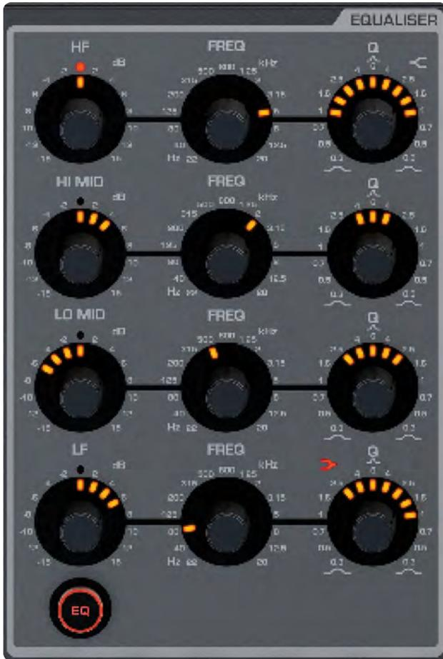
The channel EQ (Equaliser) section is used for sculpting the tonal (frequency-based) balance of the signal. The Impact EQ has four fully parametric, full range bands - LF and HF have switchable bell/shelf modes. You can check the EQ 'curve' via the Touch Screen Main Menu EQ button.
