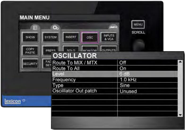
It is not possible to route directly to the console's LR and MONO buses, though you can route the Oscillator signal to a Mix bus master then use the LR and MONO routing keys.
