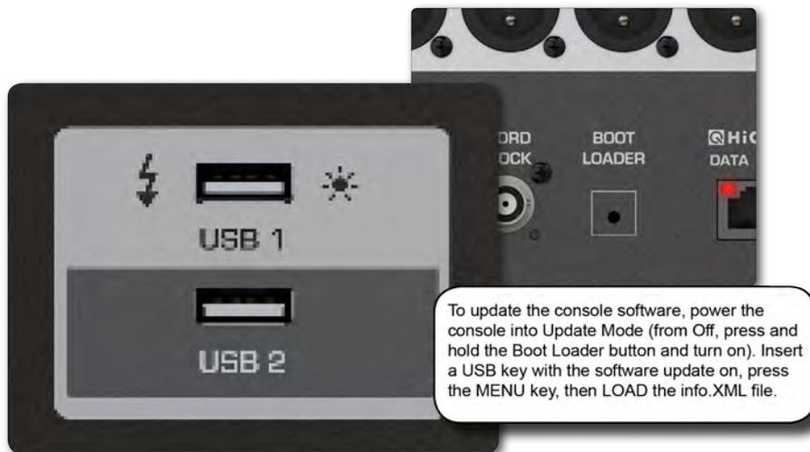
The Si Impact software is updated via the USB data port on the front panel. Details and special instructions for any release will be included with the software release package; however, the 'normal' procedure is listed below for reference:
