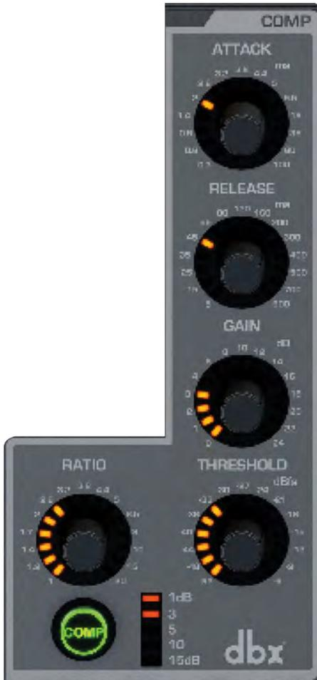
A compressor is a threshold driven process used to reduce the dynamic range of a signal by applying gain reduction when the signal level exceeds the threshold and applying 'make-up gain' to keep the overall level consistent.
