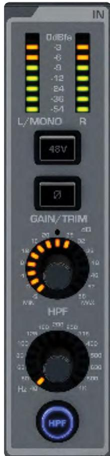
The input section mainly provides the features required for input channels such as phantom power and mic/line level. Metering is applicable to all DSP channel types, and HPF (High Pass Filter) is available in Mix Bus Master Channels.
