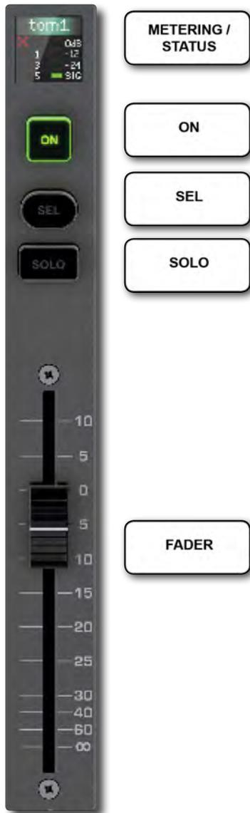
Control channels contain the primary performance controls and indicators. Layers of Control Channels (assigned to various 'actual' channels) are selected using the FADERS (Fader Layers) button group. Control channel positions are assigned to channels using the Touch Screen FADER SETUP menu (see section 3.2.1).
