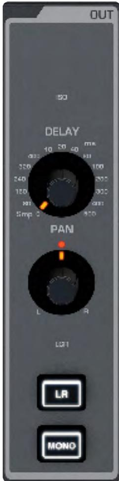
The outputs section contains features specific to the outputs of all channels. Delay and Pan (or balance) are applicable to all channel types, while LR and MONO/CENTRE routing is specific to input and Mix Bus Master output channels (not Matrix master channels).
