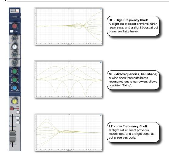
The shelving bands of the EQ (LF and HF) use a slight boost at the EQ's frequency when cutting, and a slight cut when boosting.
