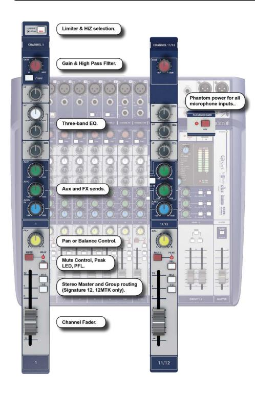
The controls are shown in the order they appear on the console channel strip - from top to bottom. This is not necessarily signal path order. Please refer to the relevant signal path diagram (section 4).
