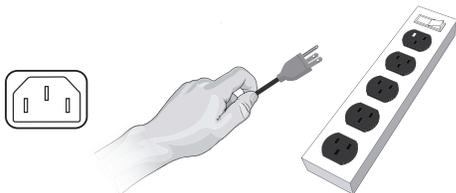
1. Connect the supplied power cord to the Blue IEC inlet on the rear of the speaker
