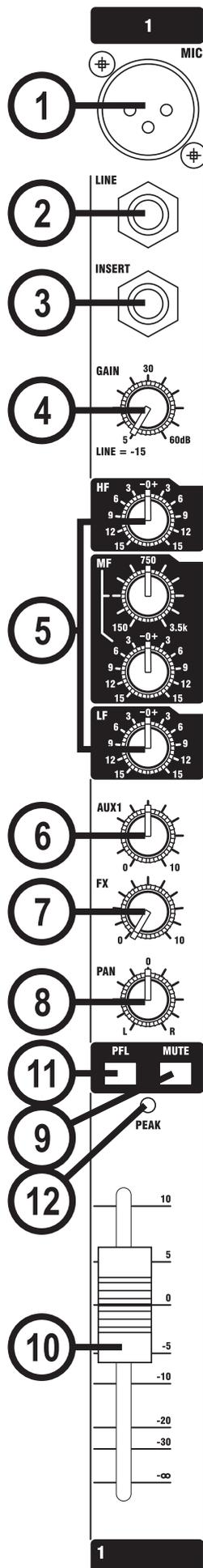
Note that some sound equipment, particularly that intended for domestic use, operates at a lower level (-10dBV) than professional equipment and will therefore need a higher gain setting to give the same output level. See “Initial Setup” on page 31 to learn how to set GAIN correctly.
