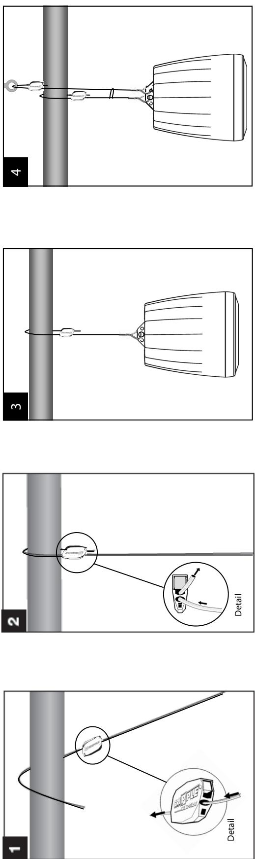
1. Thread Grapple onto cable (see inset detail). Pass over ceiling anchor point (as shown) or through other secure anchor point of the building structure. Installer is responsible for ensuring that anchor point is secure to building structure.
