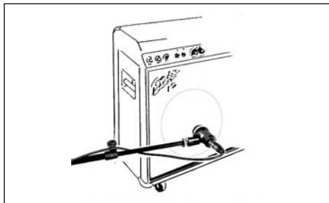
Fig. 3: Microphone placement for a guitar amp.
